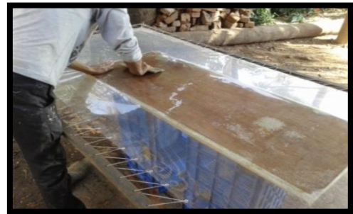
Fig8(k) Preparation of Bamboo panel
