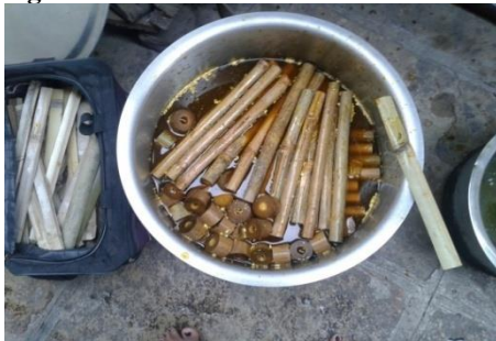
Fig. 3- Dipping Process of bamboo
